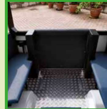
Pneumatic disabled access platform lift
