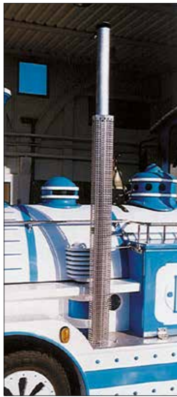
Upwards external stainless steel exhaust
